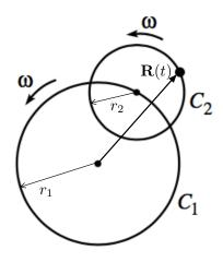
The position of the mass relative to the center of C1 is indicated by the vector  $\mathbf{R}(t)$ . Find the direction and the magnitude of the fictitious force felt by the mass due to rotations of both circles.
